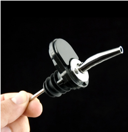
The BarVision pouring spout wirelessly sends data from its tilt and time sensors to the BarVision Controller.
